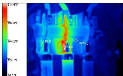
you can also change the emissivity or temperature range, to better analyze the results. That means you don't have to get the perfect image on-site, which is a big time-saver.
